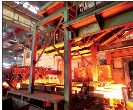
**Descaling of steel sheets and profiles.**
