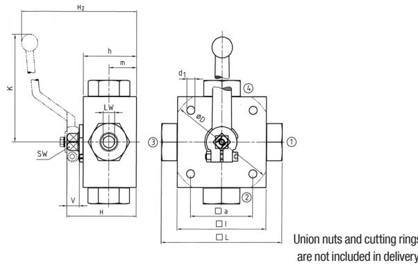
**High-Pressure Block Body Ball Valve • Type TBV-4
