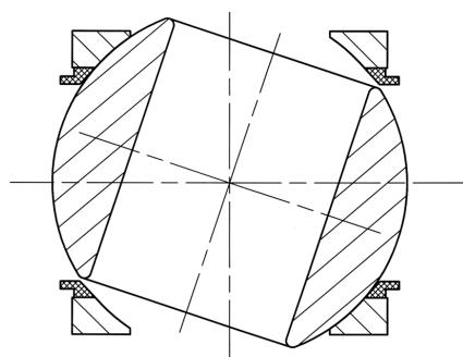
The ring is made of special material and protects the seats against erosion.
