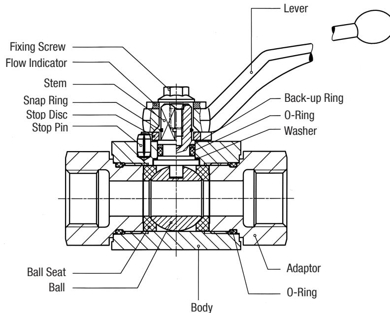
The assembly of the lever and the flow indicator has to be carried out the way that the groove of the stem and the groove of the indicator are identical in direction.
