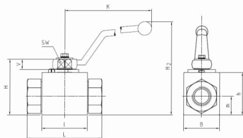
**High-Pressure Block Body Ball Valve ▪ Type BBV-2**
