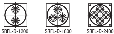
Detail arrangement of filter elements
